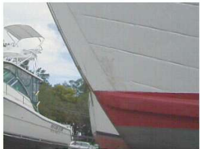
Figure 7. Views of the bow of a boat hull constructed of wooden planks. Routine maintenance involves caulking the seams between the wooden planks to prevent moisture intrusion. The infrared image confirms that caulking is needed as it shows cooler areas where moisture has entered into seams.
