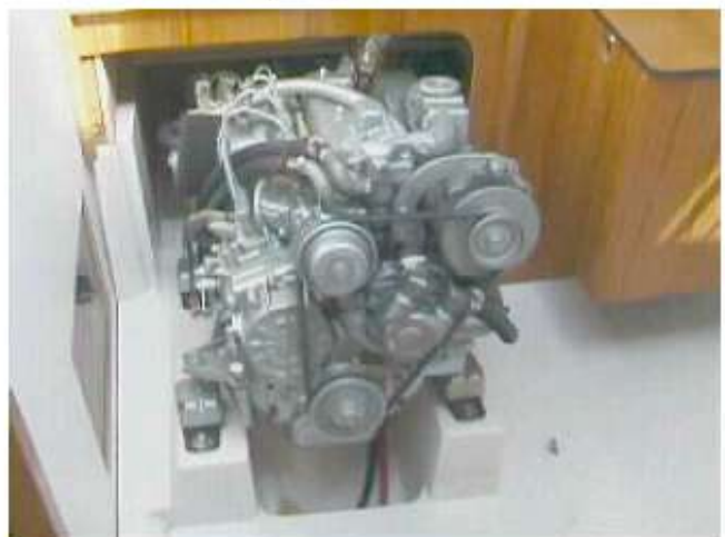
Figure 4. Views of a 3-cylinder naturally aspirating diesel engine. Visual photograph (right) shows the engine with a factory installed low amperage output 12VDC alternator. Owner replaced original "wet cell" battery bank to one with a larger capacity. The new battery bank was much too large to be effectively charged by the factory installed alternator. There were no visual signs that the alternator was being overworked, however the battery bank would never get fully charged and batteries suffered from sulfation. Infrared showed windings in alternator were hotter than expected. This visual evidence coupled with measuring low input voltage at the battery terminals solidified the recommendation why the buyer should upgrade to a higher amperage output alternator.
