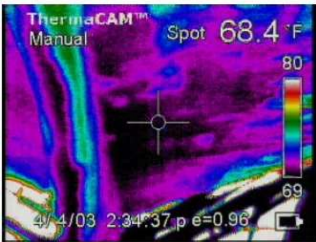
Figure 8. A common practice to extend the life of the bottom of a wooden boat is to sheath it in FRP. It is used to reduce maintenance and prevent marine organisms (e.g., Terado worms) from boring into the wood. Sometimes the physical bond between the wood and FRP breaks down, and water gets trapped in the interstitial space. The wood continues to decay and the FRP disbonds from the wood. Coolness in the infrared image shows the extent of water entrapment and disbonding that can be heard when sounding the hull with a percussion hammer.
