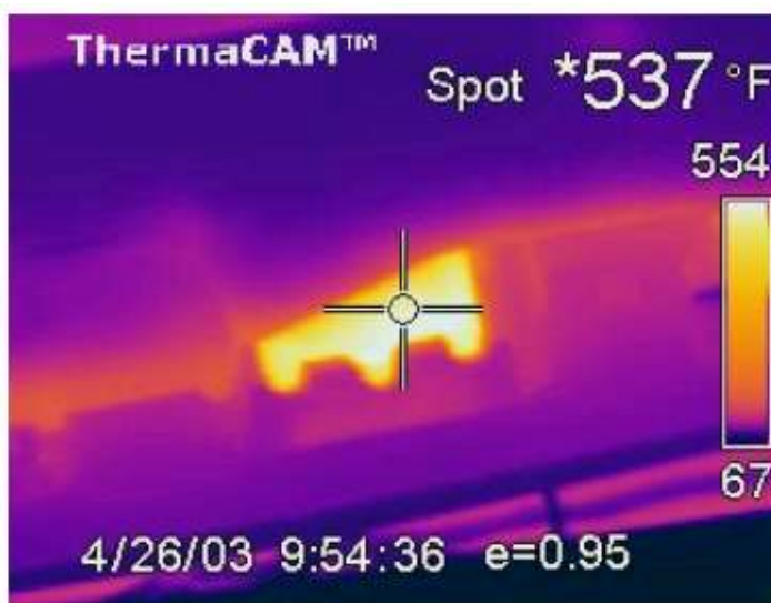
Figure 3. Views of a portion of an exhaust manifold for a 160 hp 6 cylinder turbocharged diesel engine. During the sea trial, the engine overheated. A thermal image of one of the exhaust ports on the manifold showed excessive temperature. Buyer advised to have a marine mechanic examine the turbocharger system.
