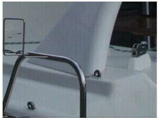
Figure 10. On deck photos of the sailing catamaran shows the exterior side corresponding to the interior ceiling. Note the raised deck in the FRP construction. It is common practice to use a composite construction to reduce the weight of the boat. In this case the composite is FRP/wood/FRP. If the raised deck area were constructed with a solid FRP laminate, it would be much heavier and cost more to construct. A lighter boat sails faster than a heavier boat.
