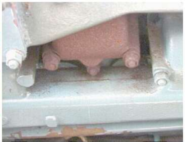
Figure 3. Views of a portion of an exhaust manifold for a 160 hp 6 cylinder turbocharged diesel engine. During the sea trial, the engine overheated. A thermal image of one of the exhaust ports on the manifold showed excessive temperature. Buyer advised to have a marine mechanic examine the turbocharger system.
